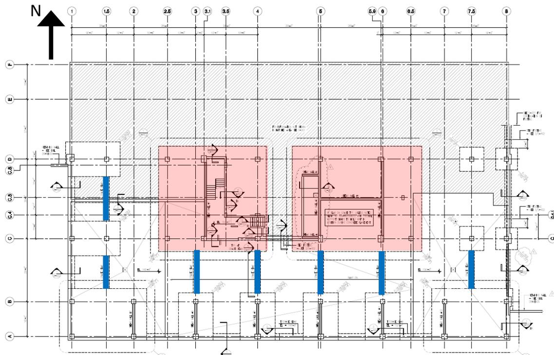
Figure 2: Foundation Plan (Level P0) Showing 48" Thick Mat Foundations Shaded in Red
